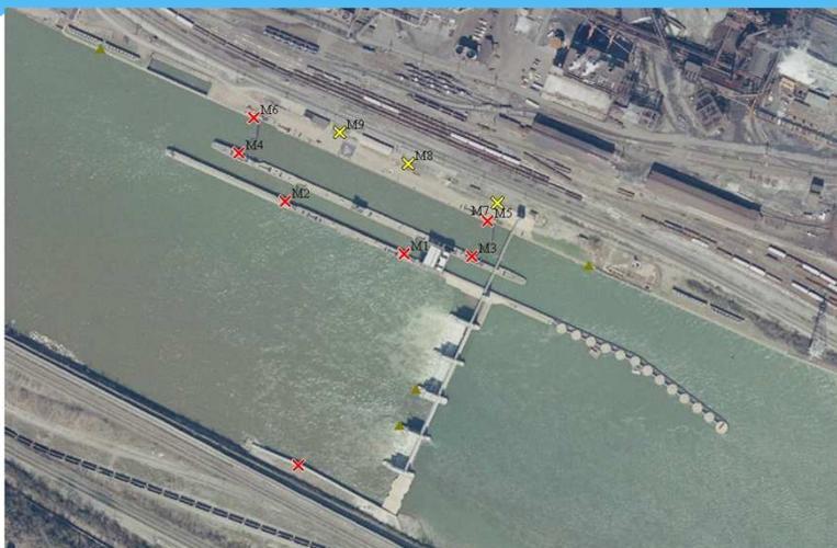
Add constraint on left bank abutment—remaining points are 4 mm
