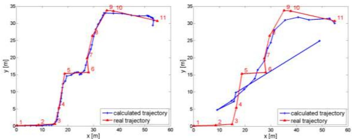
Figure 4. Results of two test runs along trajectory 2
