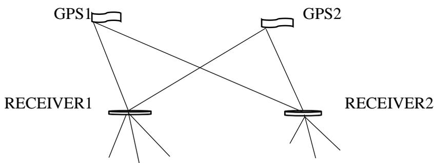
Figure 2: Double differencing; Source: Eissfeller et al. (2011)
