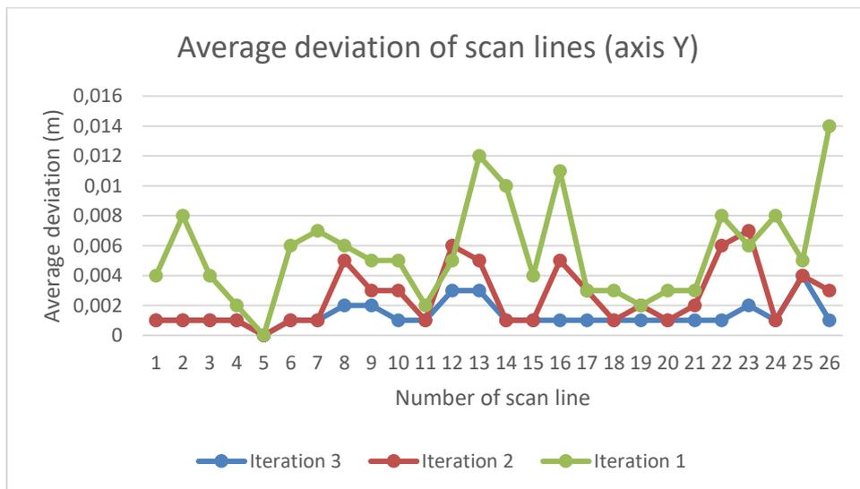
Graph 2. Average deviation values of scan lines by Y axis (1<sup>st</sup>, 2<sup>nd</sup> and 3<sup>rd</sup> iteration)
