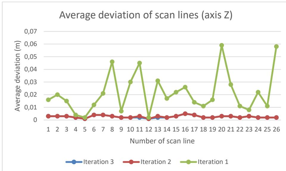
Graph 3. Average deviation values of scan lines by Z axis (1<sup>st</sup>, 2<sup>nd</sup> and 3<sup>rd</sup> iteration)
