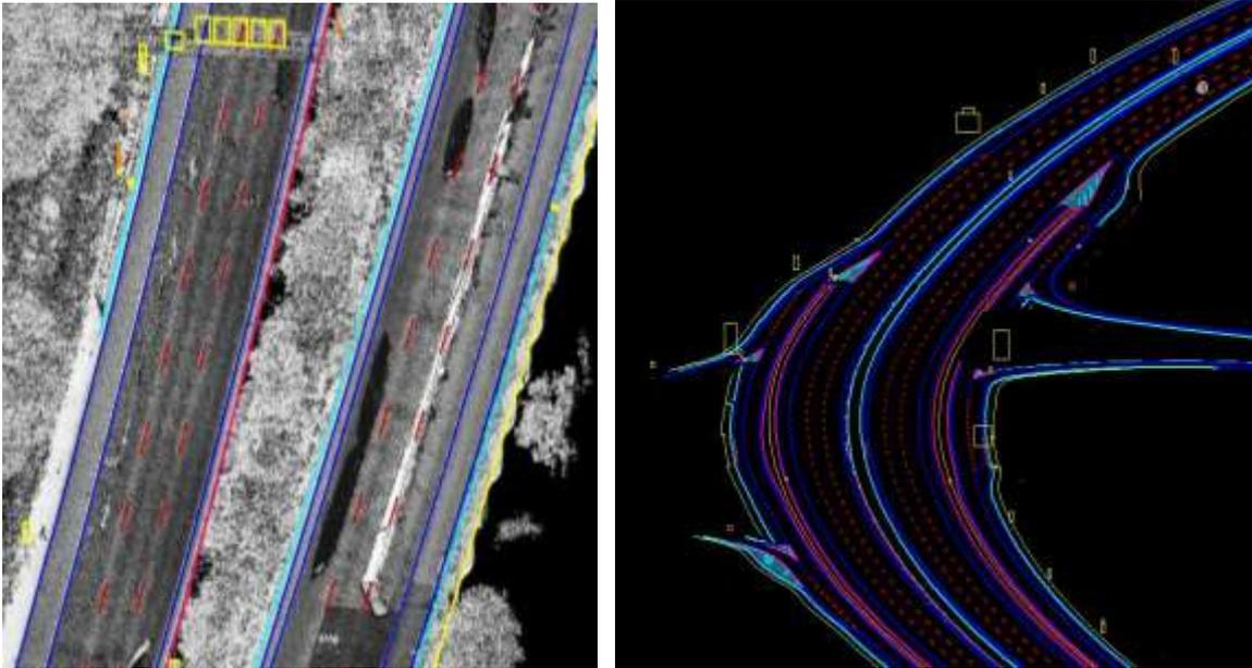
*Figure 4. Example of extraction of the road infrastructure – high way*
