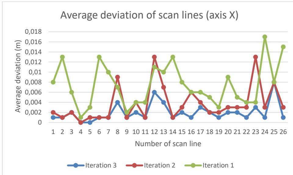
Graph 1. Average deviation values of scan lines by X axis (1<sup>st</sup>, 2<sup>nd</sup> and 3<sup>rd</sup> iteration)
