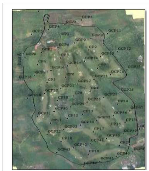
**Figure 2. GCP and ICP distribution plans**
