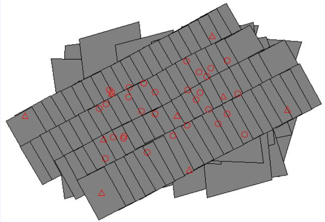
Figure 6: The combined UltraCamD and oblique Pictometry images footprint after performing AT
