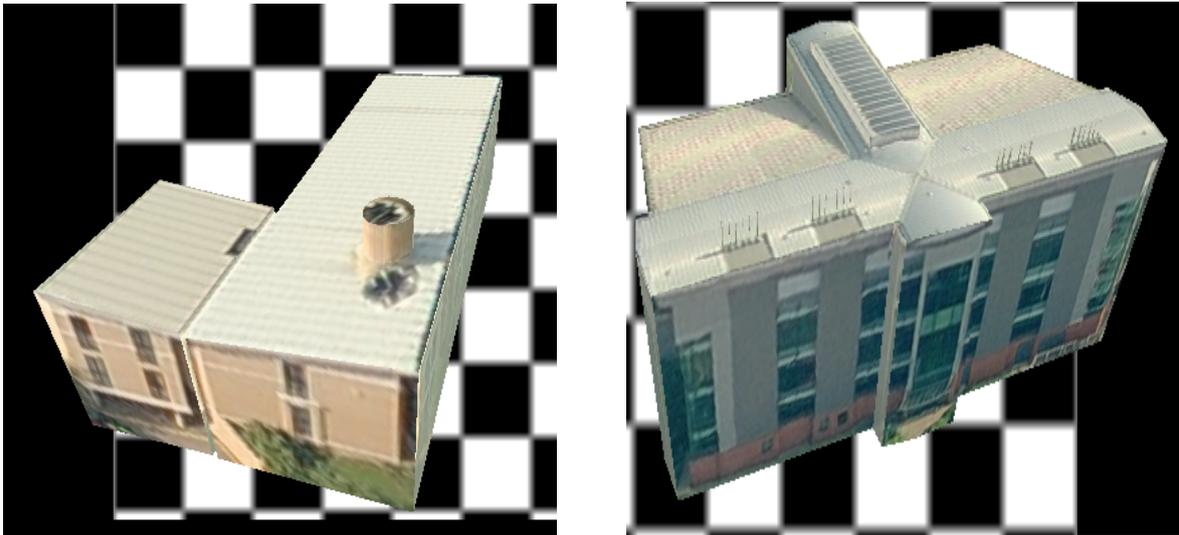
Figure 9: 3D building model textured using Pictometry oblique images block
