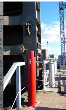
Previous Geodetic Monitoring Campaign executed by University, Geodesy Department using GPS on pillars. Control points and monitoring points on red steel pillars anchored on massive concrete foundations.
