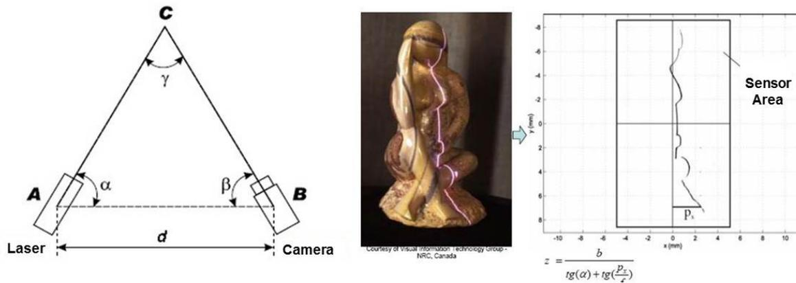
**Figure 1:** 3D object scanning by triangulation method
