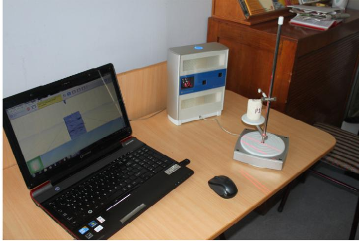
**Figure 2:** Nextengine 3D desktop scanner
